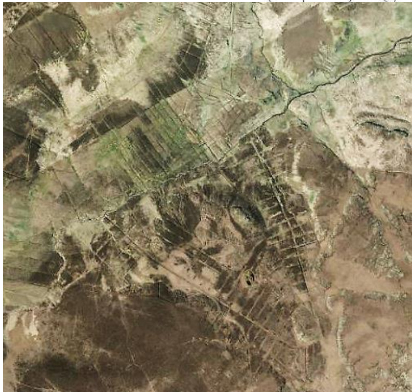
Recent aerial photo of the peat works showing layout of former lines used to transport cut peat to the aerial ropeway – steam engines hauled wagons. The mechanism driving the aerial ropeway is not clear but presumably relied on a combination of gravity and some powered mechanism at the lower station
